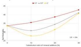
Figure 06 : Evolution of the shear threshold according to the mineral addition
