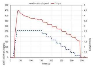
Figure 04: Evolution of torque (T) and rotational speed (N) as a function of time
