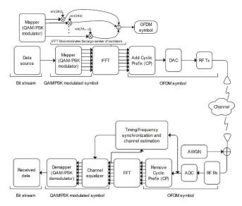
Figure 1: Block diagram of transmitter and receiver in an OFDM system.
