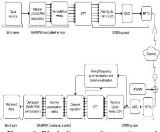
Figure 6: Block diagram of transmitter and receiver in the proposed OFDM system.
