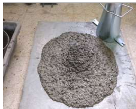
Figure 7. Slump flow test for fresh HPFRFC mixes.
