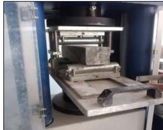
Figure 9. Flexural strength test for hardened HPFRFC mixes.
