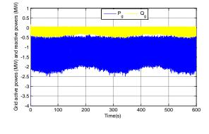
Figure 10. Grid active and reactive power.
